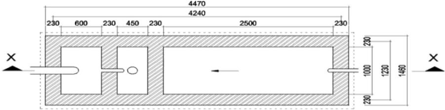
**SECTIONAL PLAN OF THICKENING TANK**
