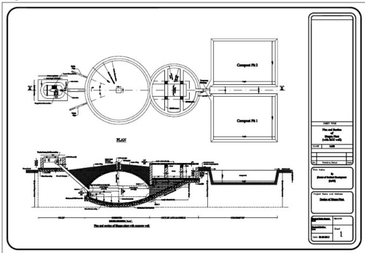
Figure 3: Schematic Diagram of the Proposed Biogas Technology
