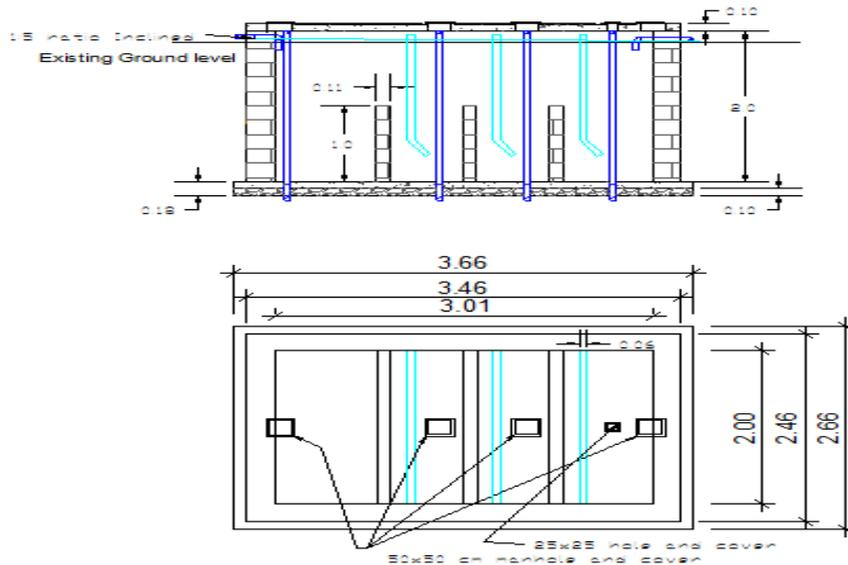
Figure 4: Schematic Diagram of Dewatering System (Sludge thickening unit)
